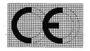
The CE marking must have the same vertical dimension and may not be smaller than 5 mm. If the CE marking is reduced or enlarged, the proportions given in the above drawing must be respected.
